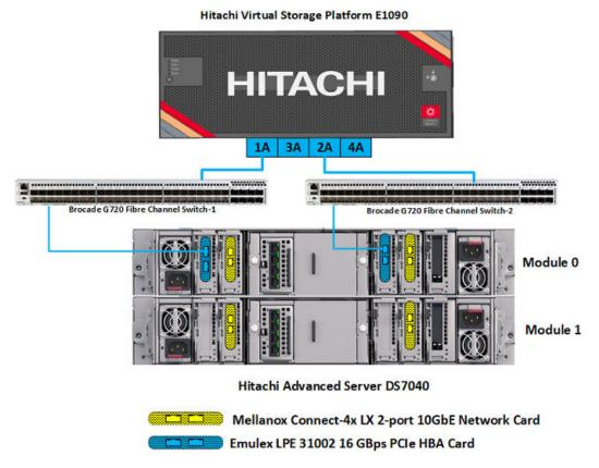
Each Hitachi Advanced Server DS7040 server has two 2-port Emulex LPE31002-M6 16 Gbps PCIe HBA cards on the Master Module (0), PCIe slot 0, slot 2.
